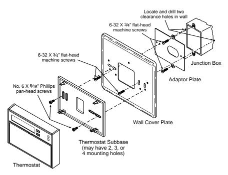
Figure 2. Mounting 1F9X digital thermostat to vertical junction box
